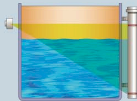
Liquid Continuous Level Measurement with Source and Detector Mounted Externally on the Vessel
